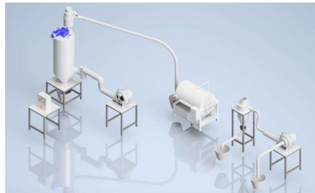
Figure 2. Completely machine of dust separator process
