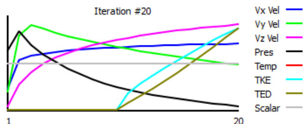
Fig 10. Convergence plot graph of the airflow distribution of a mortar grenade with a fin inclination of 2.5° from its axis.
