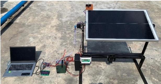
**Fig 5.** Testing Of The solar power plant Dynamic Two-Axis Tracker System and Data Collection Using A Data Logger
