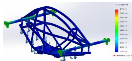
Fig. 9. Stress Value at 1300 N Load
