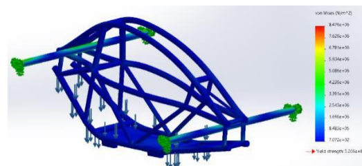
Fig. 9. Stress Value at 1300 N Load
