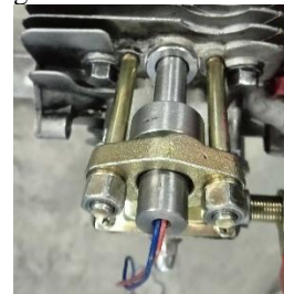
Fig. 4 Thermocouple Sensor Setting
