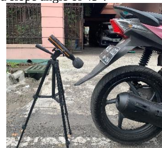
Fig 2. Decibel meter installation
