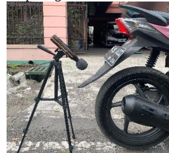
Fig 2. Decibel meter installation
