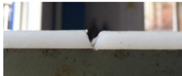
Figure 3. Root Face Height Preparation
