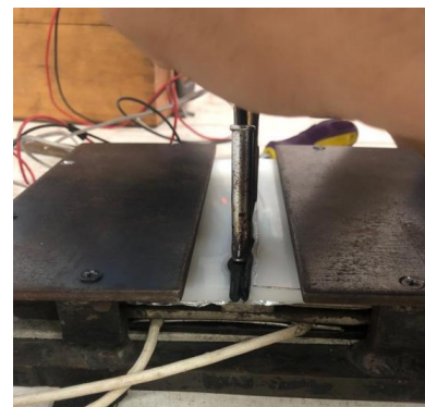
Figure 4. Specimen Welding Process with HWG
