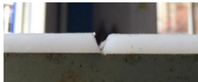
Figure 3. Root Face Height Preparation
