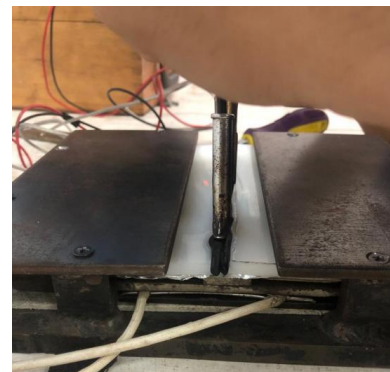
Figure 4. Specimen Welding Process with HWG
