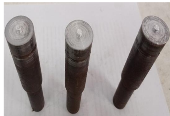
Figure 3. Tool double side friction stir welding
