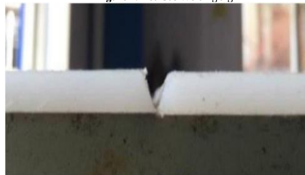
Figure 3. Preparation of the V-Groove
