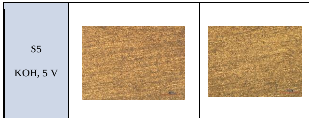
Fig 8. Images of anodic oxide films formed on titanium using Potassium Hydroxide
