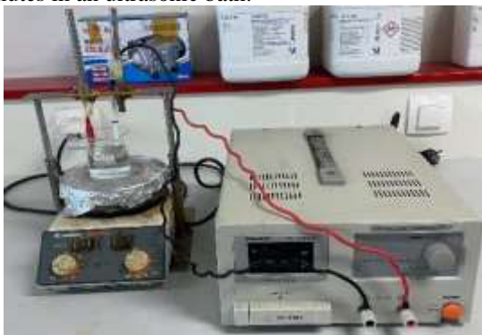
Fig 6. Anodizing set up
