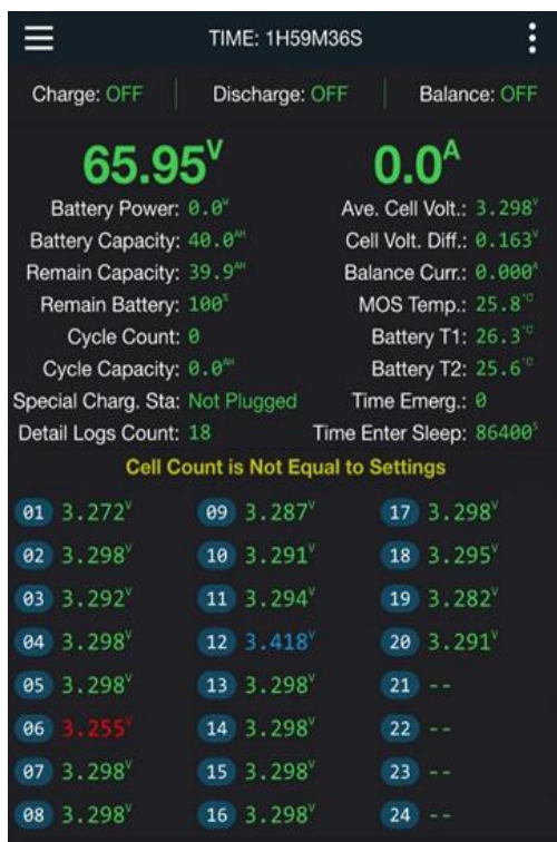
Fig. 10. Test results when Battery Management System is on Standby
