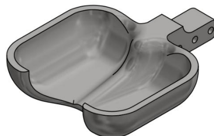
Figure 7. Pelton turbine bowl.
