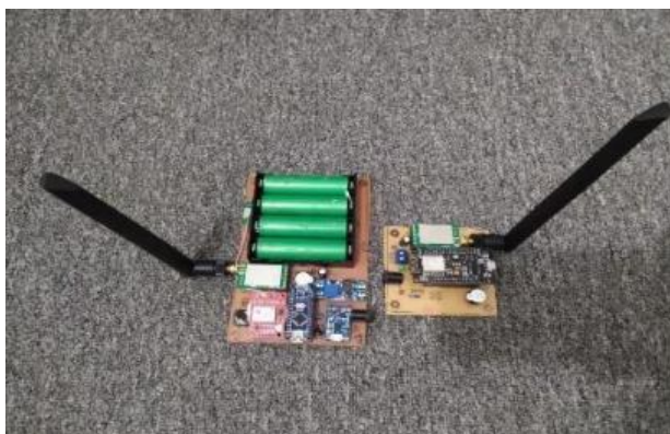
Figure 5 Design of Receiver and Transmitter Box
